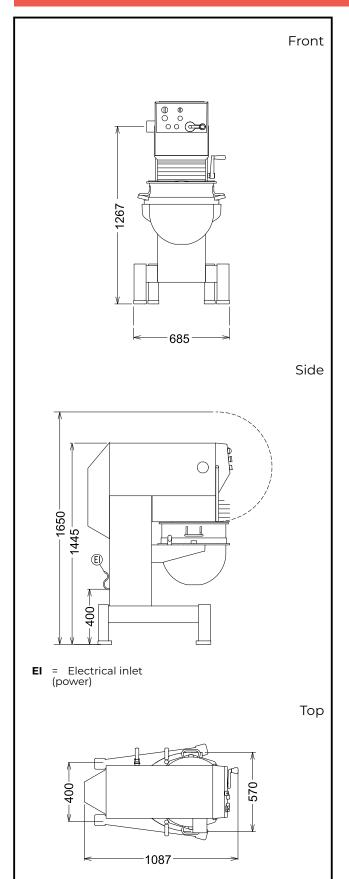
Electric 220-240/380-415 V/3 ph/50 Supply voltage: **Electrical power max:** 1.54 kW **Total Watts:** 1.54 kW Capacity: ISO 9001; ISO 14001 kg/ Performance (up to): Cycle 60 litres Capacity: Key Information: External dimensions, 685 mm Width: External dimensions, 1087 mm Depth: External dimensions, Height: 1445 mm **Shipping weight:** 332 kg ISO 9001; ISO 14001 kg with Spiral hook **Cold water paste:**
